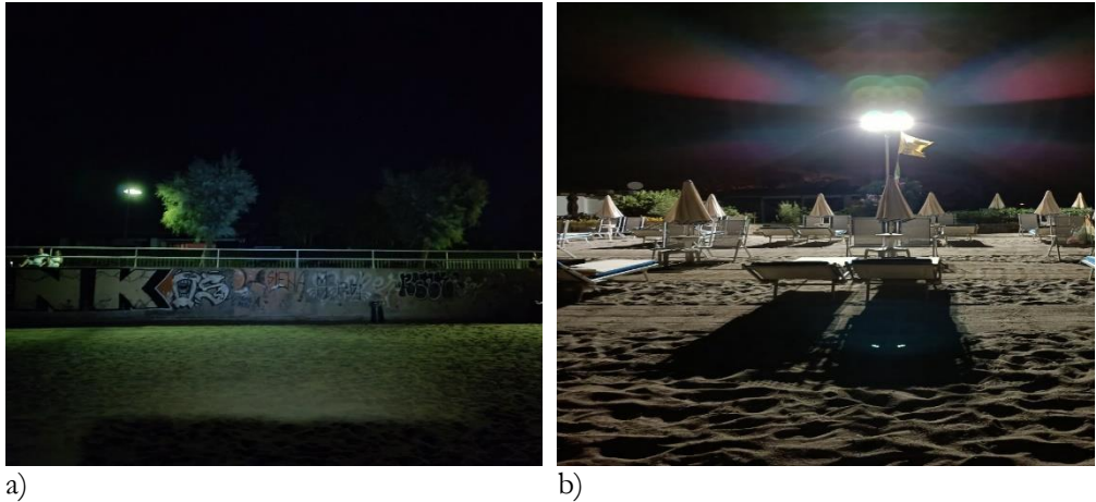
Fig. 6 – Light source with proper direction of the light beam (best) and right light intensity to illuminate a promenade by the sea (a). Light source with evident incorrect direction of the light beam (worst) and excessive light intensity produced on a beach a night (b)
