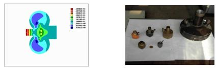
Fig. 5. Static pressure function (Re=1,000, Eu =10). Fig. 6. Types of mixer atomisers
