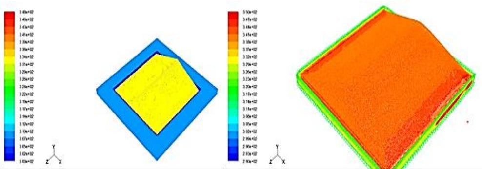
Figure 7. Temperatures in the glass cover. Images made in the Fluent program, de la compañía ANSYS [www.ansys.com], (scale in °K).
