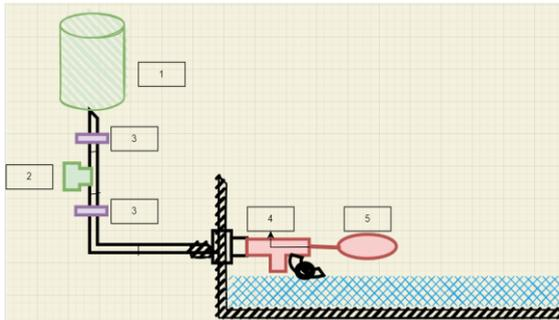
Figure 3. Detail of the location of the float concerning the solar still: 1) Saltwater container, 2) Container shut-off valve, 3) Union nuts for container separation, 4) Water level control valve, 5) Float for opening/closing of the water inlet valve.
