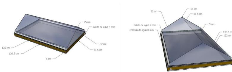
Figure 4. A side and front image of the double slope solar still design
