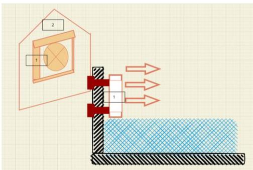
Figure 2. Solar still in operation with forced convection: 1) Fan, 2) Vertical wall for fan support
