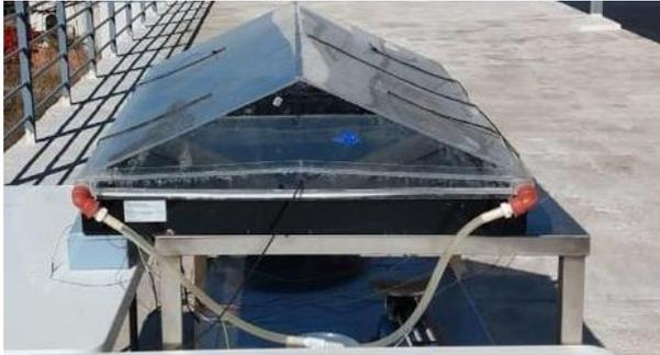
Figure 1. Solar still in operation
