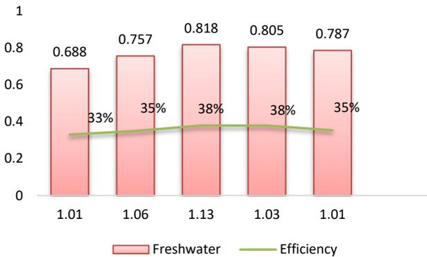
Figure 9. Freshwater production as a function of solar energy received in the solar still.
