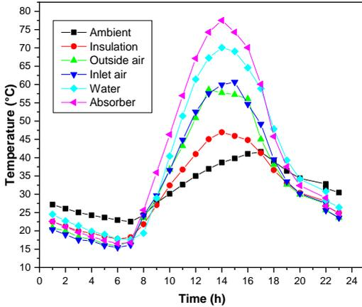
Figure 6. Temperatures inside and outside of the solar still.
