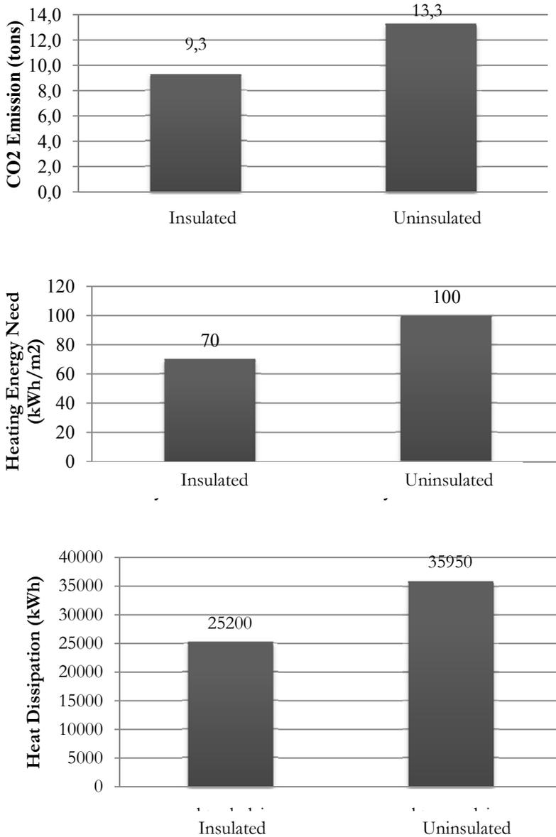
Figure 4. Insulated and uninsulated condition of buildings
