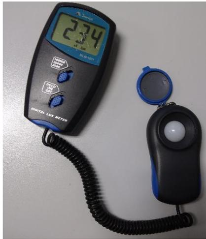
Fig. 1. Portable luxmeter used for measurements.
