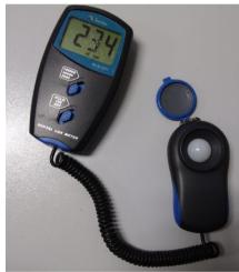
Fig. 1. Portable luxmeter used for measurements.
