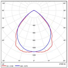
Fig. 3. Luminous intensity distribution curve for the lamp-luminaire assembly chosen.
