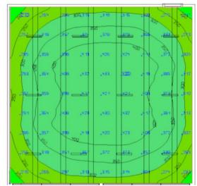
Fig. 5. Illuminances on the desk plan of room A obtained from the Dialux software
